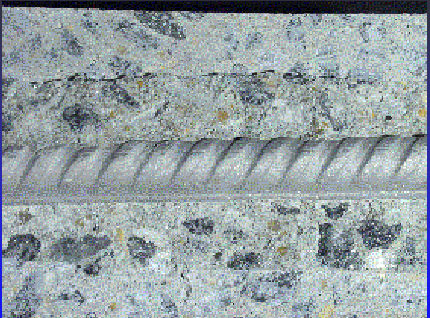
A Pickled 316L Stainless Steel-Clad Bar
