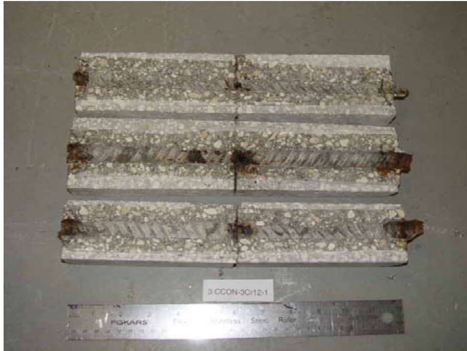
Figure 4.85. Photo. Trace of the upper rebar and corrosion products on specimen number 1-CCON-3Cr12-1.
