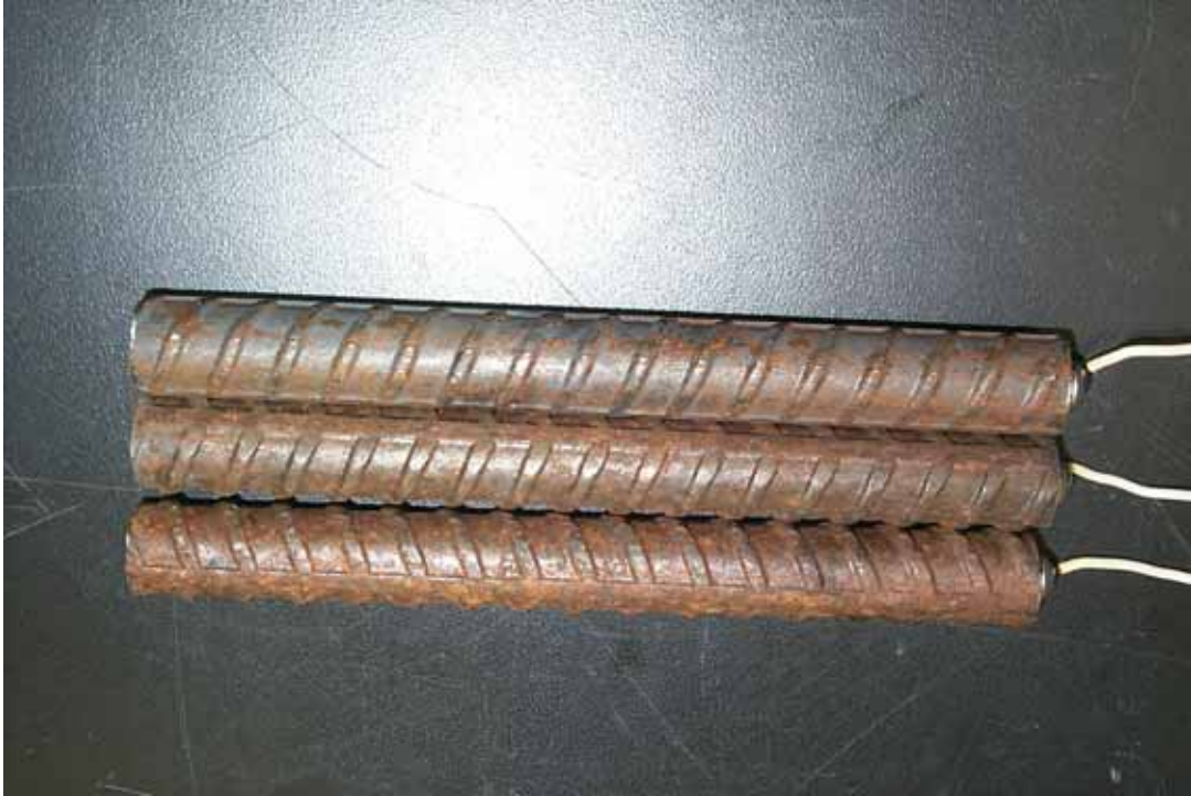
Figure 4.12. Photo. Type 2201 SS specimens subsequent to AST-1 testing.
