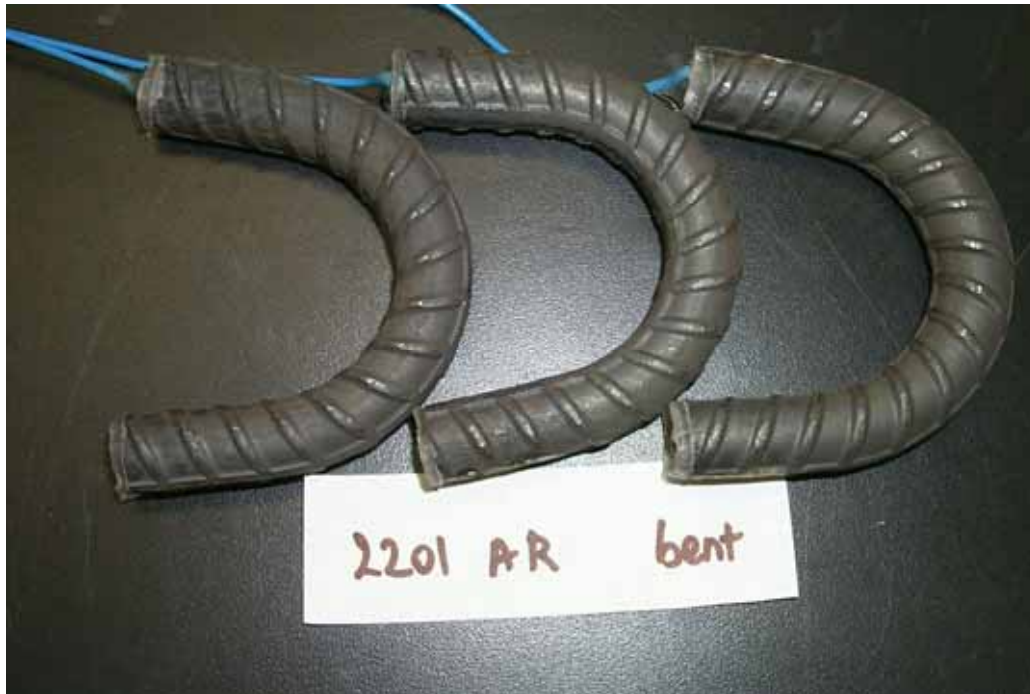
Figure 3.2. Photo. Three bent, as-received Type 2201 stainless steel bars with electrical leads.
