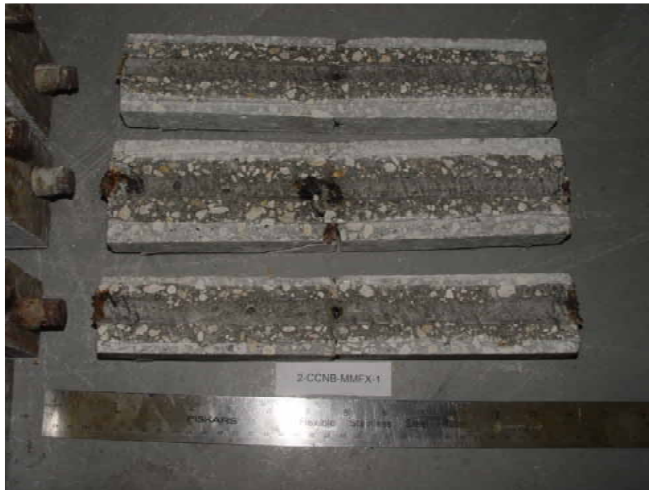
Figure 4.64. Photo. Trace of the upper rebars and corrosion products on specimen number 2-CCNB-MMFX-1.
