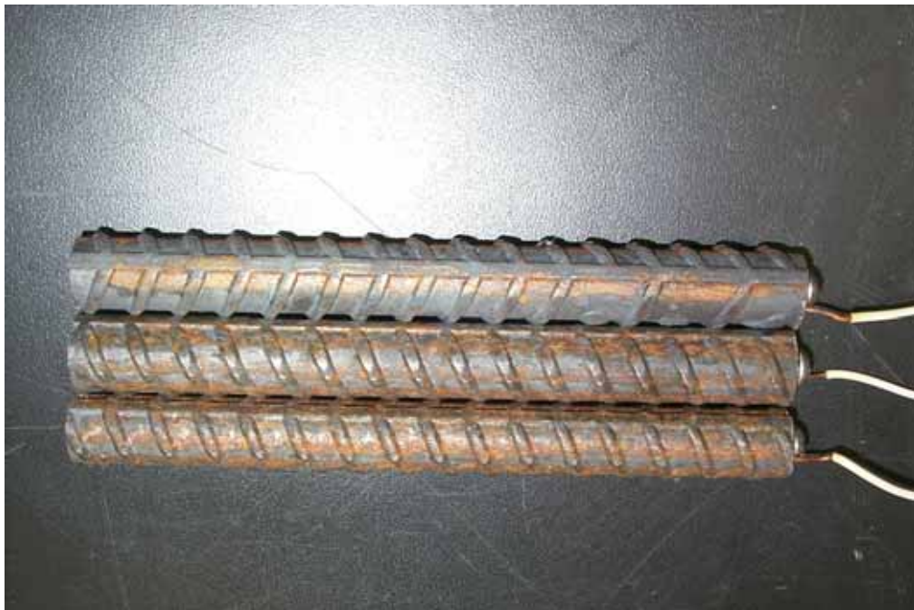
Figure 4.11. Photo. Type 2205 SS specimens subsequent to AST-1 testing.
