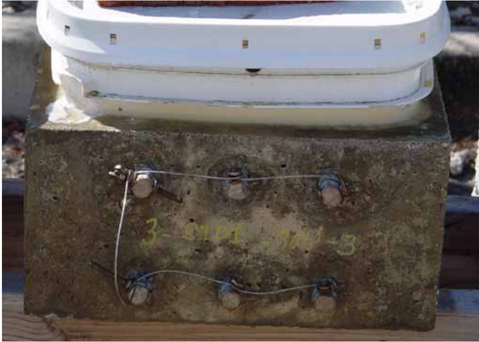
Figure 3.19. Photo. Ponded deck slab specimen under test.
