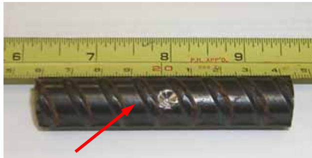
Figure 3.4. Photo. Damaged MMFX-II™ specimen.
