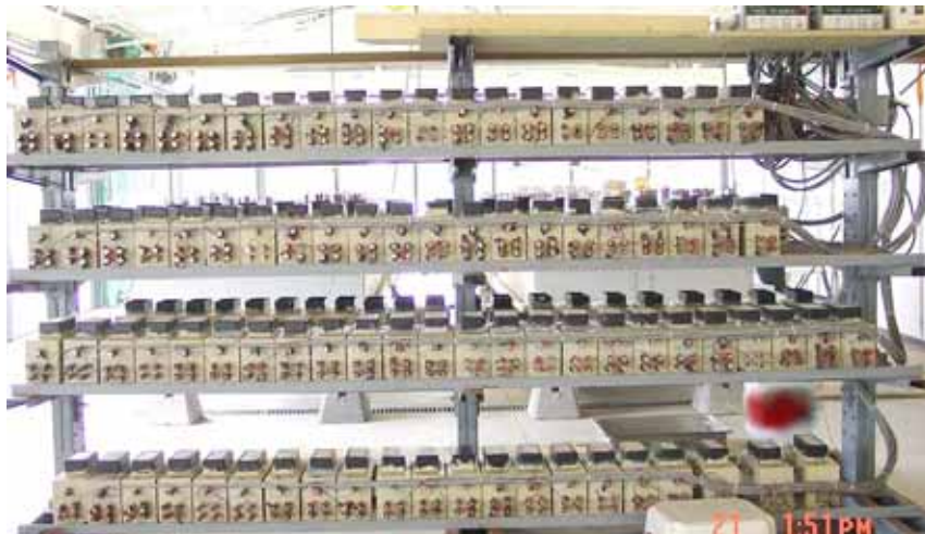
Figure 3.25. Photo. Macro-cell slab specimens under exposure.
