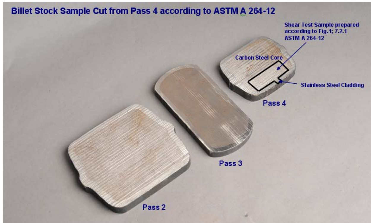
Figure 1. Showing location of shear test sample (photo supplied by Cladinox)
