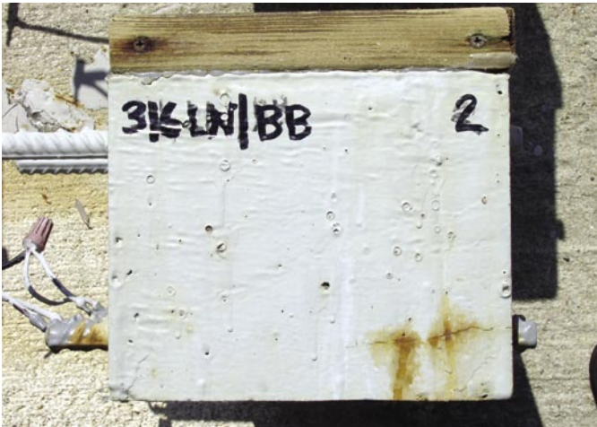
Fig. 4: Side view of a concrete block with 316LN bars at the top and CS bars at the bottom
