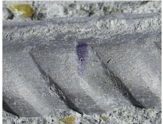
Fig. 14: One of the holes (marked area in the center) drilled through the cladding of a 316L-clad bar. Notice the absence of any sign of corrosion around the hole, even though it was apparently not filled with cement paste
